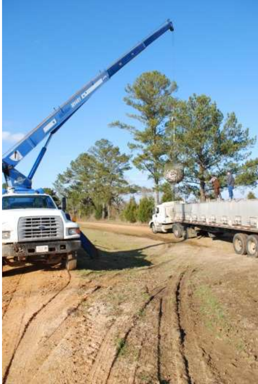
Figure 9. This boom truck can lift and move heavy loads of fish from ponds to live haul trucks. Boom trucks are regarded as being much safer than backhoes because the boom can be moved more slowly and precisely than a backhoe boom.
