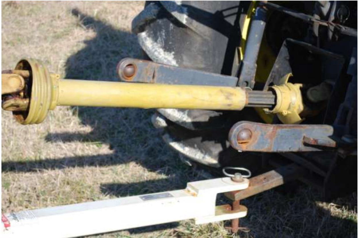
Figure 27. Power take-off (PTO) shields prevent workers from becoming entangled in the spinning PTO. Severe injuries and fatalities can be prevented by the use of a PTO shield. This PTO shield is cut near the tractor to allow for lubrication to be applied. The farm owner recommended that PTO shield manufacturers provide a way to lubricate the PTO shaft without having to remove the shield.
