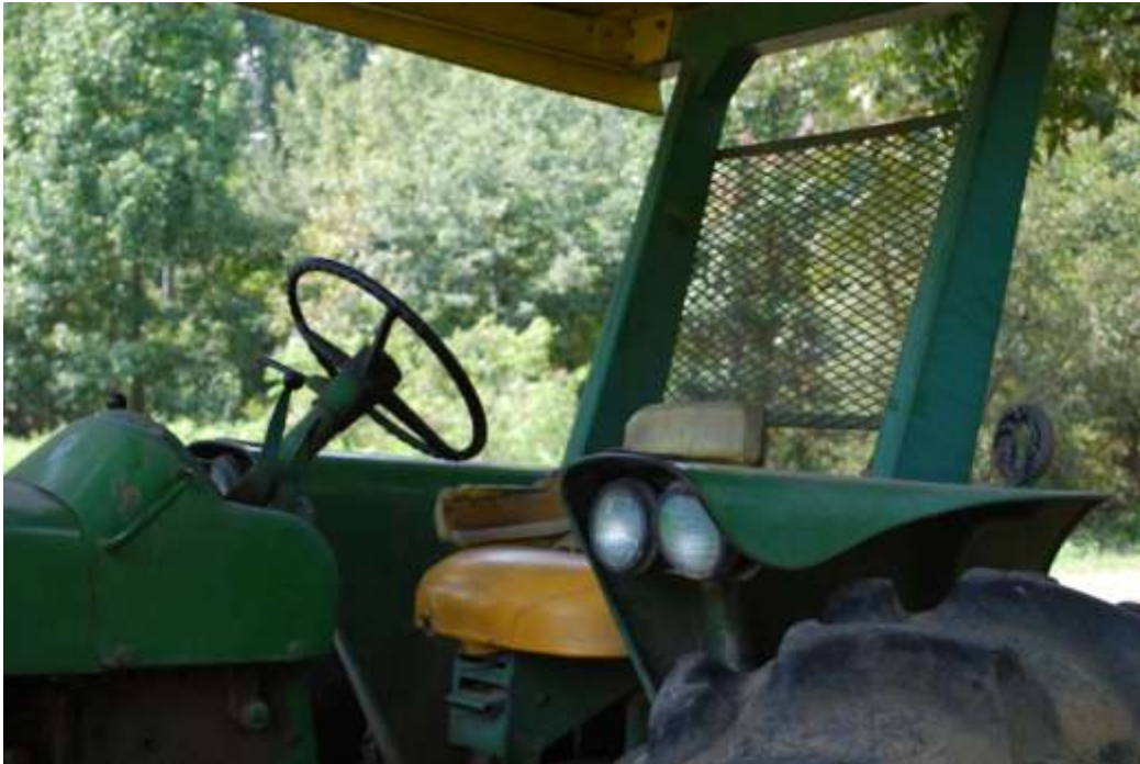
Figure 36. The metal screen welded on the tractor ROPS protects the driver from stones “launched” by a bush hog mower toward the back of his head. Such a screen would have helped a Missouri farmer who was pulling a log behind his tractor; the front of the log collided with and was blocked by a stone, causing the back of the log to flip up and strike the driver’s back. This paralyzed the man from the waist down.
