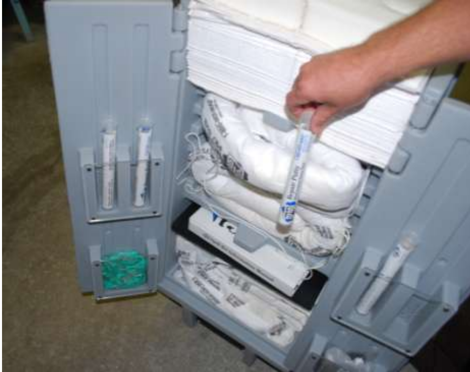
Figure 58. This chemical spill cabinet contains absorbent towels and “snakes” as well as sealant/glue to plug leaks in containers.
