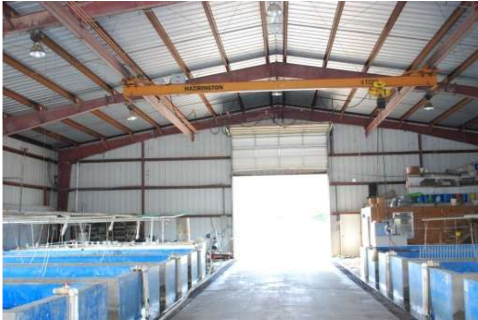
Figure 1. The overhead crane in this photograph can move heavy loads of minnows between tanks and onto live haul trucks.
