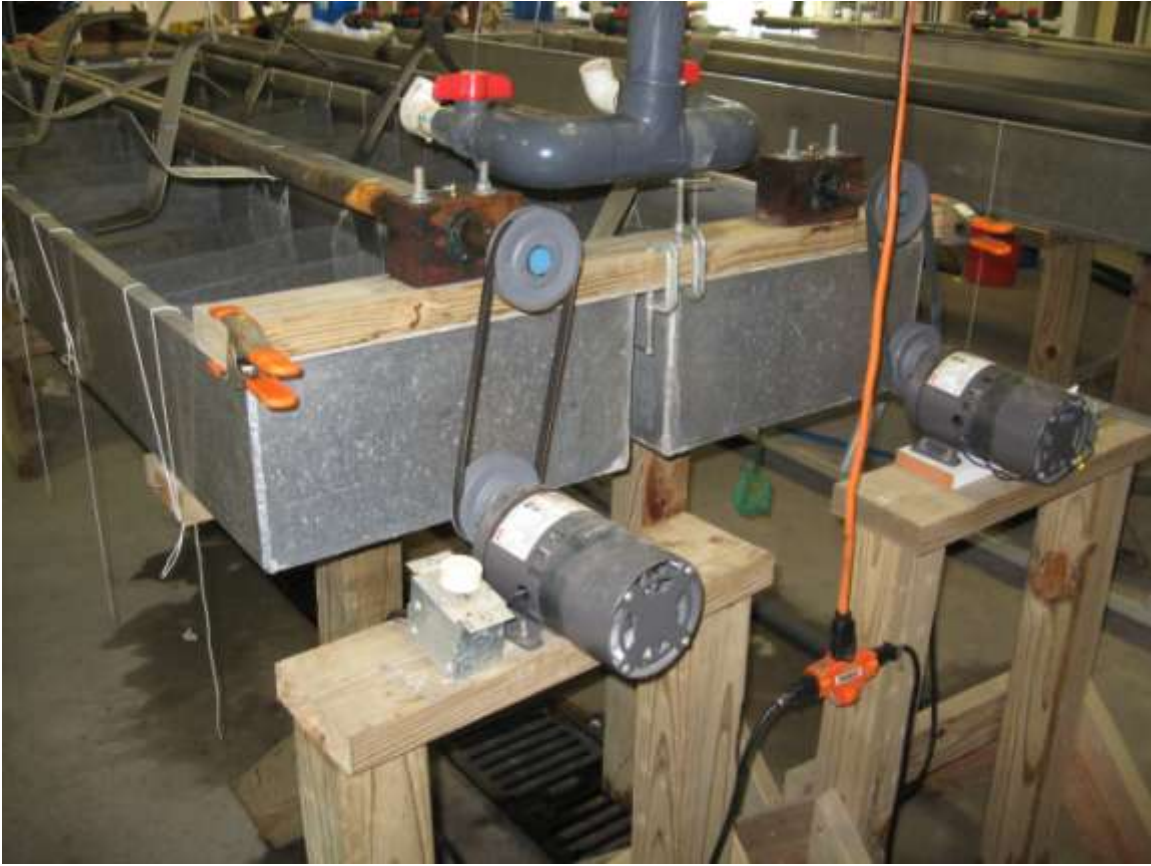
Figure 33. Catfish egg hatching troughs pose a safety hazard from the rotating metal paddles that keep the water circulating and the eggs moving. The paddles on this hatching trough will stop rotating if someone blocks them or gets caught in them; the belt on the motor simply slips and the motor is sitting on a movable, unattached sawhorse/support table.
