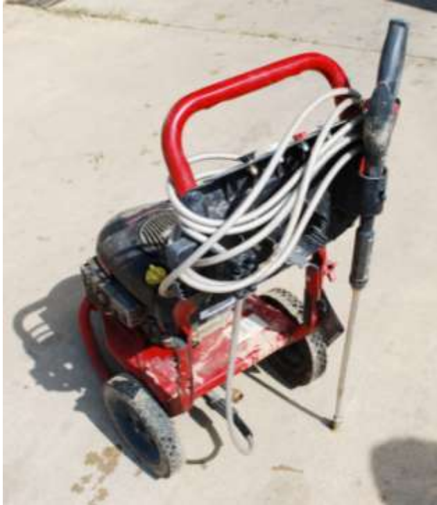
Figure 50. This farm uses only gas-powered pressure washers. This is due to a fatal electrocution that happened in July 2002. One of the farm owners was pressure washing farm equipment when a bare wire in the washer's starter capacitor came into contact with the metal lid covering the capacitor. This happened while he was holding the wand in both hands across his chest and standing in a water puddle. The insulation covering the capacitor wire had eroded away from years of vibrating against the metal capacitor lid (the lid and whole capacitor were permanently enclosed and were not designed to be checked and maintained; it appears to be a flaw in the washer's design that allowed the wire to be eroded during normal use).
