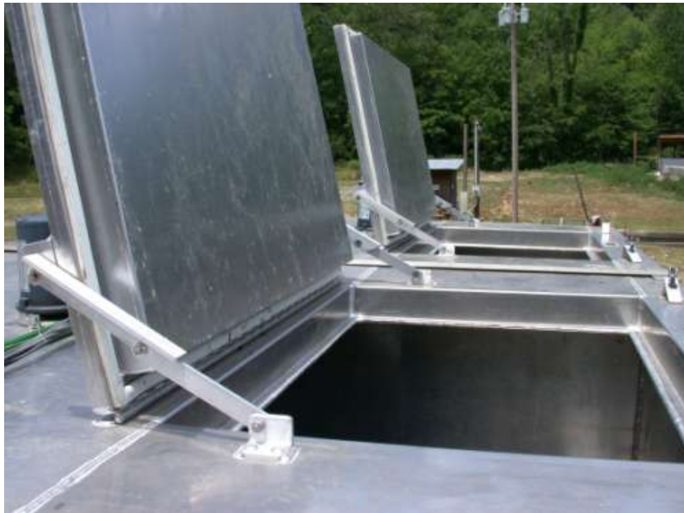
Figure 32. Locking hinges on hauling tank lids prevent them from being blown closed onto workers' hands. Other techniques for keeping tank lids open include using wedges, bungee cords and screw-down clamps.
