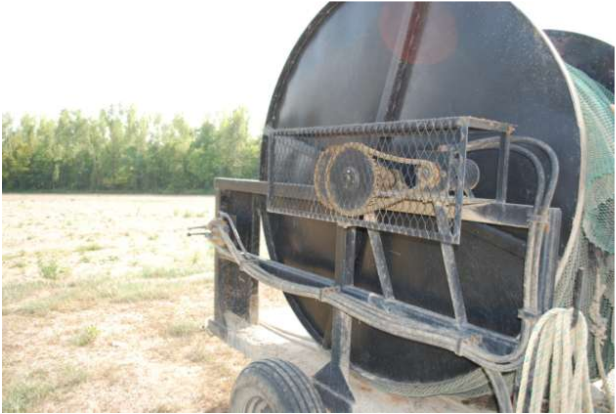
Figure 30. The gears and chain operating seine reels should be covered with a protective shield/screen. Use of a seine reel prevents muscle strain from pulling the seine by hand.
