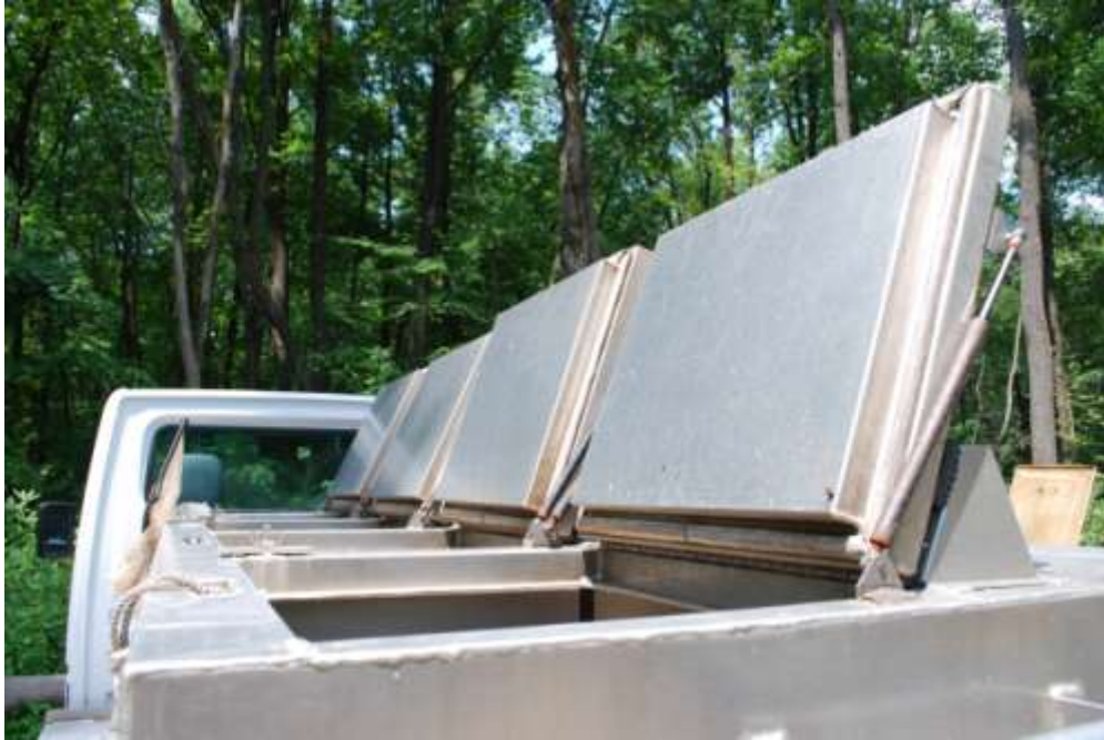
Figure 31. Gas-filled shocks can be used to prevent hauling tank lids from being slammed shut by the wind onto workers' hands.
