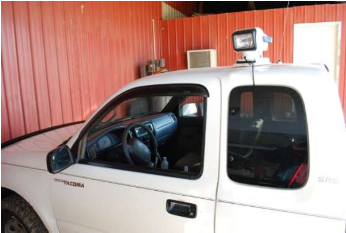
Figure 60. Spotlights mounted on trucks make nighttime work safer.
