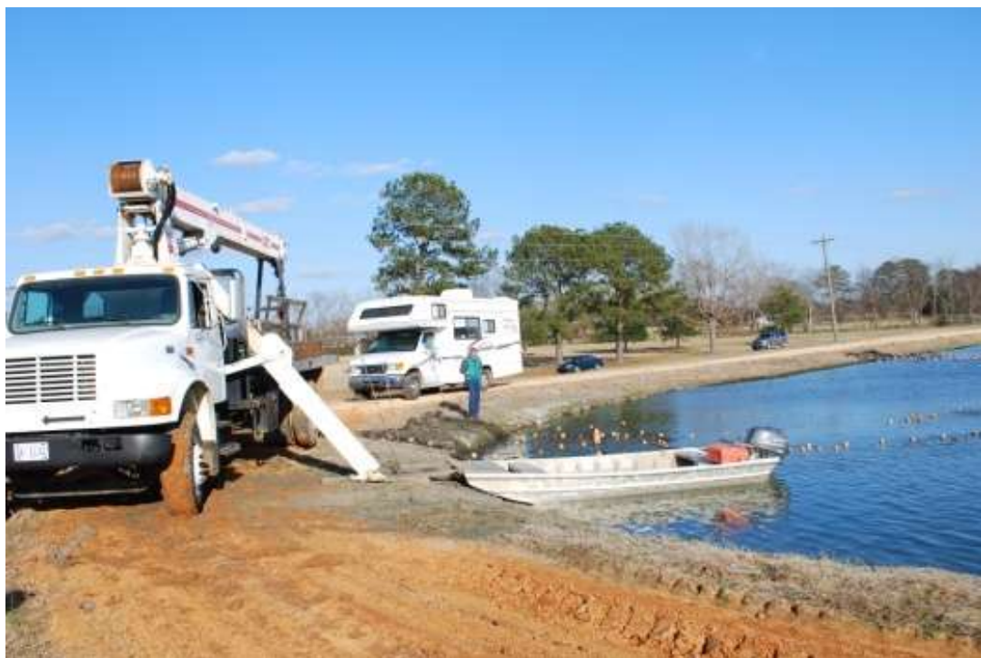
Figures 10 and 11. Boom trucks are loaded with a seine and John boat for traveling from pond to pond during harvest. The boom truck sets up on pond banks and unloads the seine and John boat for harvesting.
