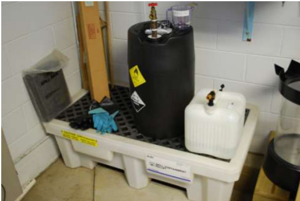
Figure 59. A hydrogen peroxide (H 2 O 2 ) container sits on a chemical spill containment platform. It is used with Argentyne (povidone iodine) to treat eggs for fungus and is replacing the use of formalin. Fumes from formalin probably pose more of a health risk for fish farm workers compared to H 2 O 2 and Argentyne.
