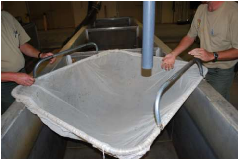
Figure 13. Two-handled dip nets spread out the weight of fish loads between two workers and prevent muscle strain.
