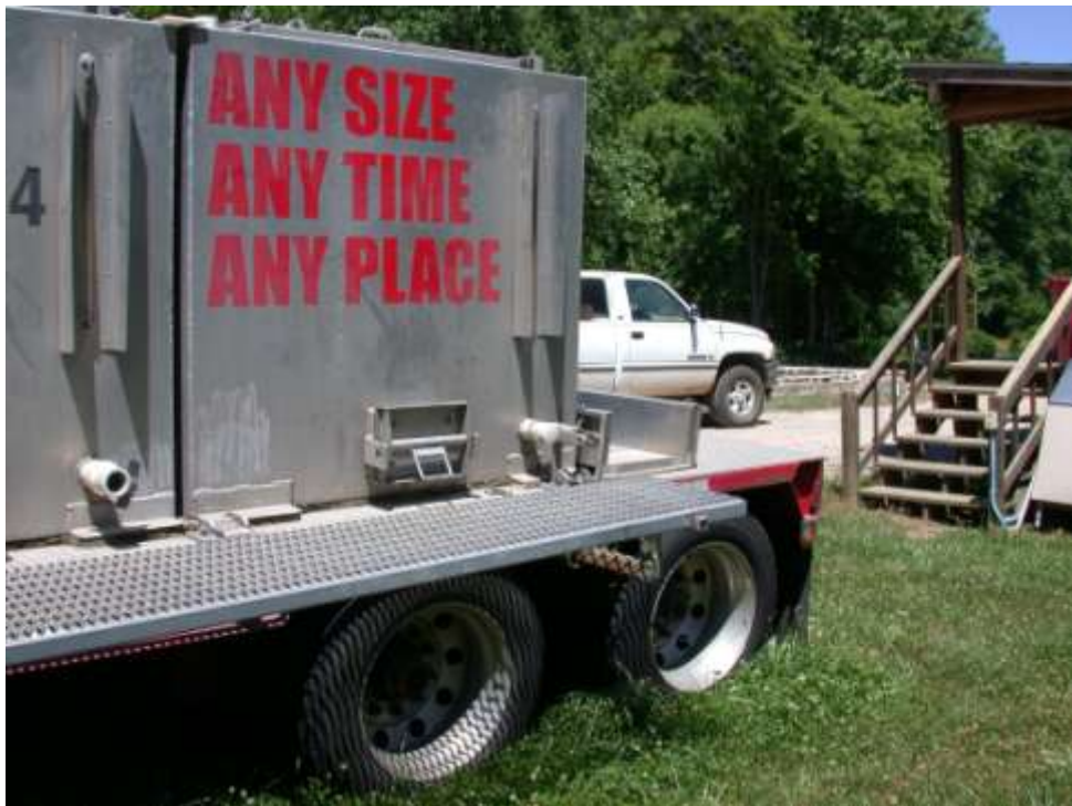
Figure 26. Metal platforms/walkways on the side of hauling trucks provide a stable work area that helps to prevent falls. They can be folded up when the truck is in motion.
