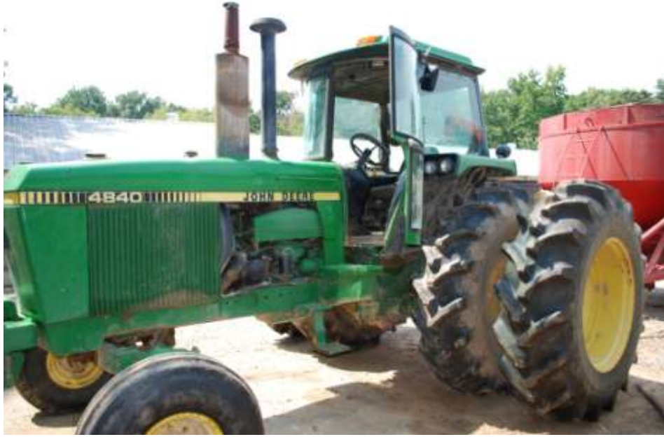
Figure 39. Tractors with double rear wheels and front wheel drive (4WD) are more stable for mowing on steep levee banks. This enclosed cab acts as a ROPS and prevents injury during tractor rollover especially when a seatbelt is worn. It is important to note that the door on the cab is on the left; if a tractor with a cab is used to mow a pond levee, the door should be facing away from the pond water because in a tractor overturned onto its right, the driver would still be able to escape from the door. Side-arm mowers pulled behind a tractor are correctly oriented to lower the blade down the levee slope on the tractor's right hand side.
