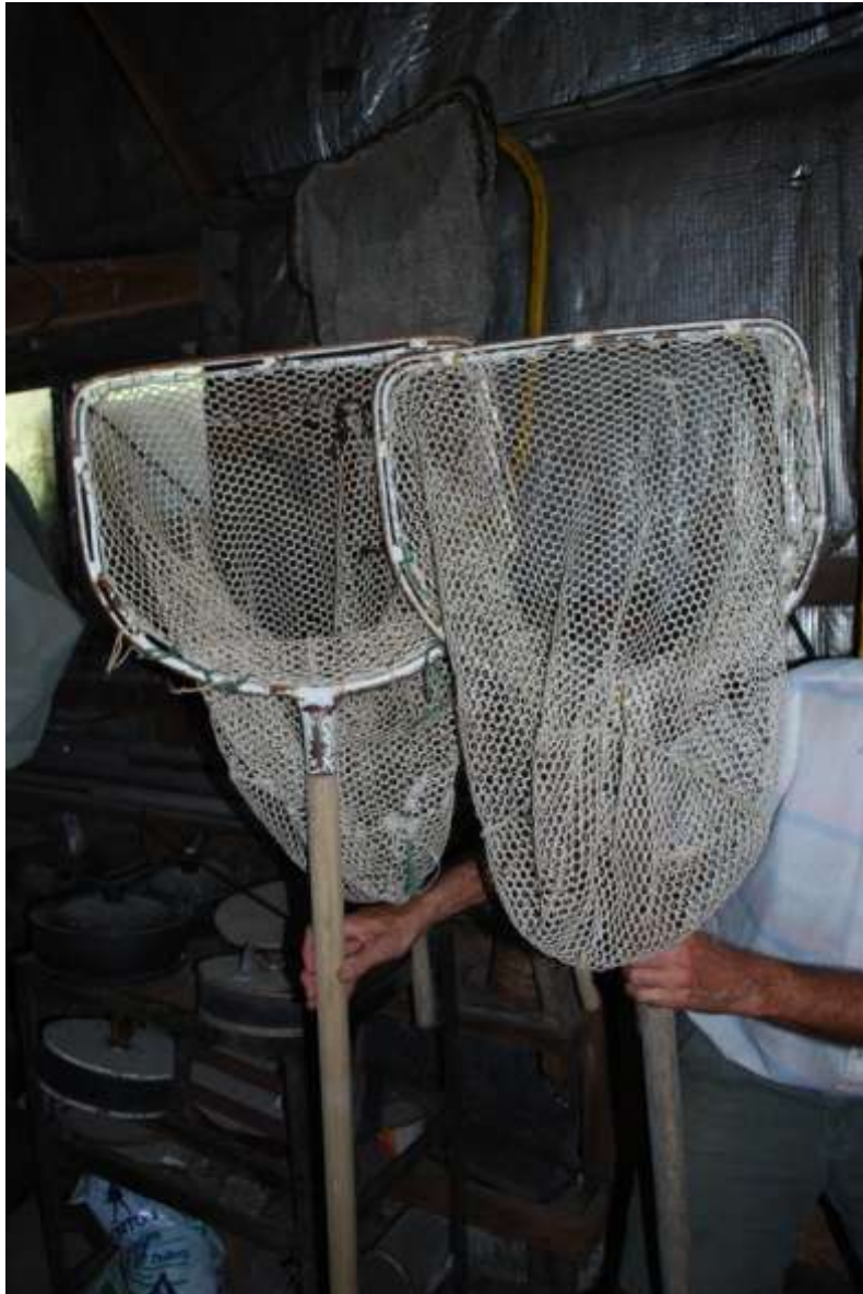
Figure 14. Dip nets should be deep enough to prevent fish from falling out when a reasonably heavy load is carried, but they should not be an excessive depth that would encourage workers to dip up a load of fish heavy enough to cause muscle strain. Dip nets that are 15 inches deep work well to meet these criteria.
