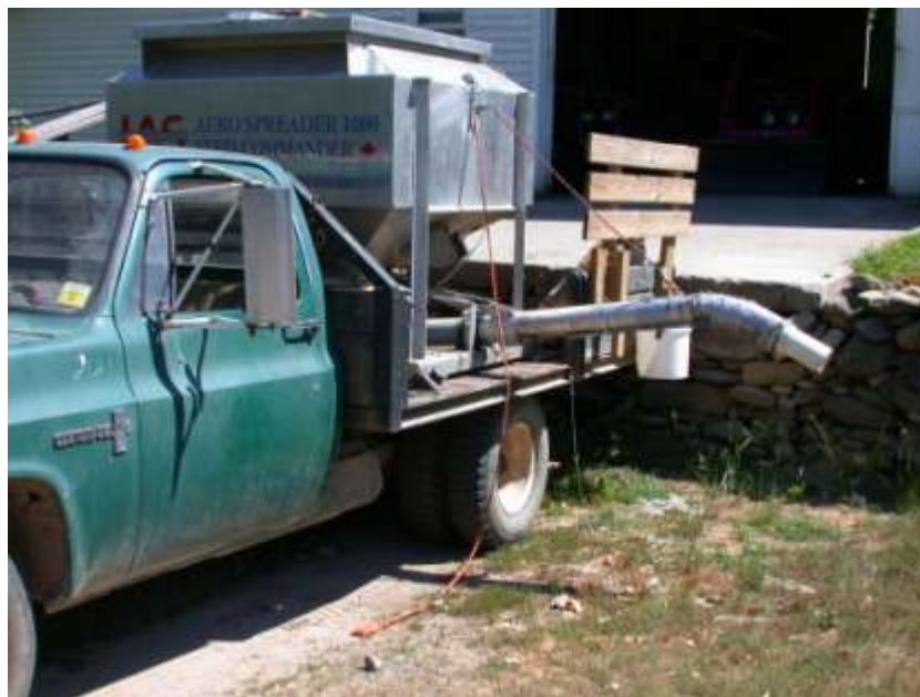
Figure 22. Feed trucks eliminate the need for manual feeding.
