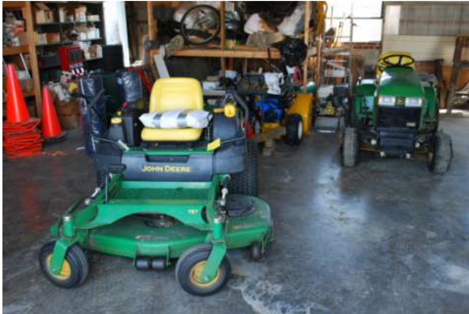
Figure 41. The “zero-turning-radius” mower on the left is designed to mow from side to side (laterally) on a hillside to prevent roll-over. The tractor mower, on the other hand, should be driven up and down the hill to prevent roll-over. Both should have roll bars.
