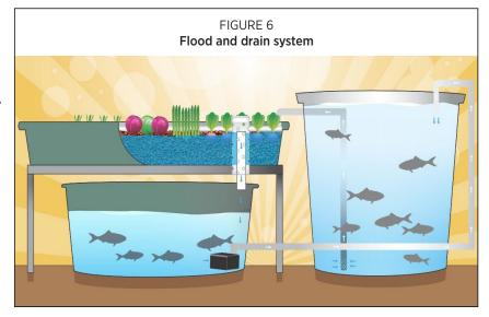
then drains back to the sump (or fish tank) drawing oxygen into the substrate for plant roots and nitrifying bacteria. The media bed supports the plant as it grows and serves as a solids and biological filter (Figure 6). Due to relatively few components and ease of construction and operation, these systems are popular for
