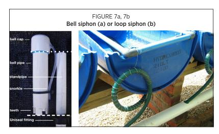
automatic bell siphon (Figure 7a) or loop siphon (Figure 7b). In both siphon methods, the pump runs continuously, controlling how fast the bed fills and drains. Fox *et al.* (2010) gives comprehensive, step-by-step instructions for building, operating, and troubleshooting an automatic bell siphon.
