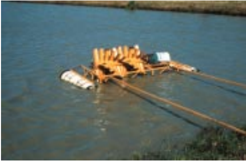
Stationary floating paddlewheel aerator.
